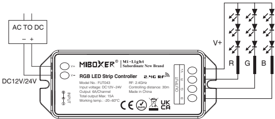
Controller connect to RGB LED strip diagram
